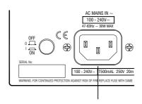
4 Connect AC mains power. Check first that the correct mains lead with sealed plug suitable for your local supply has been provided with your console. Plug into the AC MAINS IN socket making sure the connector is pressed fully in.
