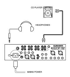
Set all controls to their starting condition. Set all **FADERS** (rotary and linear). LEVEL. AUX. RESONANCE, LFO DEPTH, HEADPHONES and BOOTH MONITOR controls to minimum. Set EQ controls to their detented centre position. Set all press switches to their up position. Set all toggle switches to their centre position.
