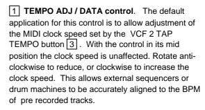
An internal jumper can be reassigned to change the function of this control to a dedicated DATA send, and will output Control Change **CC94**. See Service Options for details.
