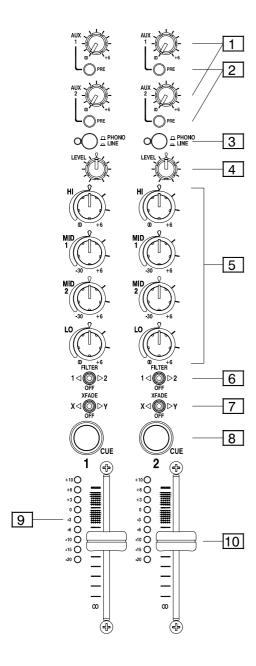
AUX 1-2 sends. Adjust the levels of the channel signals to the stereo Aux outputs. Turn fully anticlockwise to turn the signal off, fully clockwise for a maximum +6dB boost.
